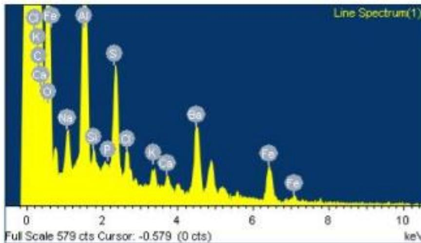
**Figure 1.** Spectrum of characteristic x-rays gathered from focusing on the thin layer of Maxon CRS coating left on the sample. Height of the peaks represents the intensity of the spectrums, and is used to determine the atomic percentage of the different elements in the material.
