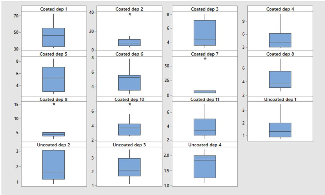
**Figure 3.** Box plots of the coated and uncoated samples at an accelerating voltage of 5kV. The coated sample at depth 7 (coated dep 7) has an unusually high carbon content for one of its replications because it detected a contaminant such as dust on the surface of the metal.
