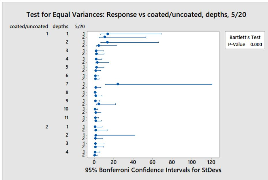
**Figure 4.** Test for equal variances. This test failed, so a 3-way ANOVA test was unable to be performed. However, this table is a good visualization of the large amount of variation shallow depths (1 and 2). Depth 1 is the Maxon CRS, and Depth 2 is 70 microns into the surface of the metal.
