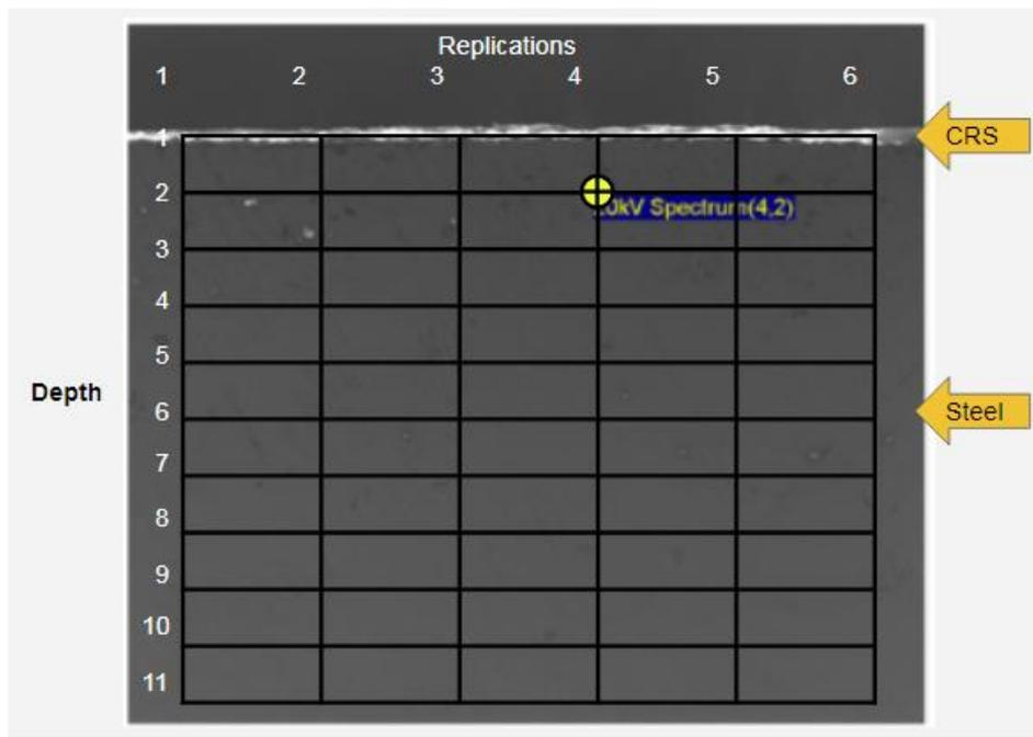
**Figure 2.** Array of points of interest that the electron beam was focused on. 11 depths, separated at a distance of about 70 microns were observed. For each depth, six replications were measured at different points. This figure has a yellow cross-hair symbol indicating that the electron beam was focused at point (4,2). This translates to replication 4 for depth 2.
