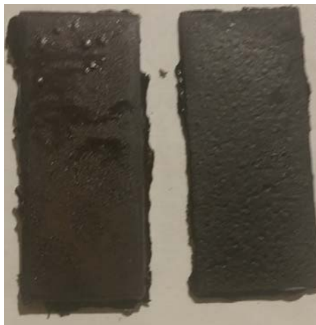
Figure 11. Day 5: Clean (left) and rusted (right) specimen before submergence
