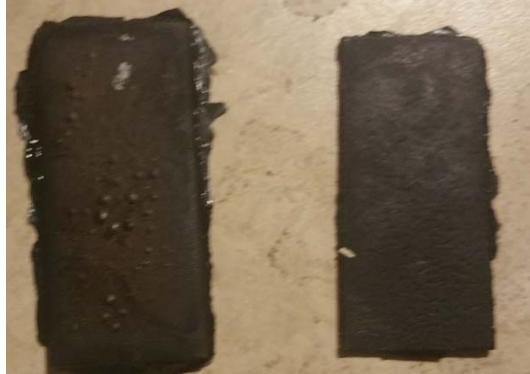
Figure 3. Day 1: Clean (left) and rusted (right) specimen before test
