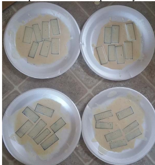
Figure 2. Seven clean and seven rusted cut pieces coated with Maxon
