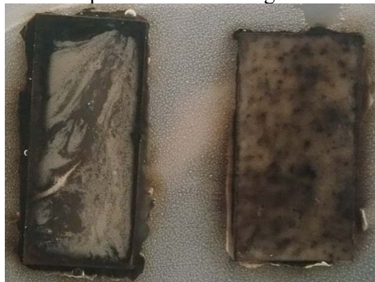
Figure 9: Day 3: Clean (left) and rusted (right) specimen at moment of submersion
