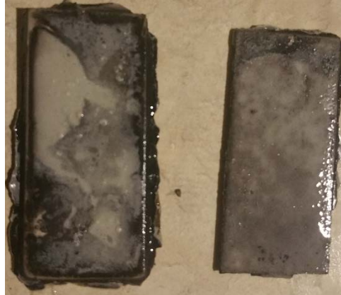
Figure 4. Day 1: After last cycle's 30 sec. submergence under warm tap water.
