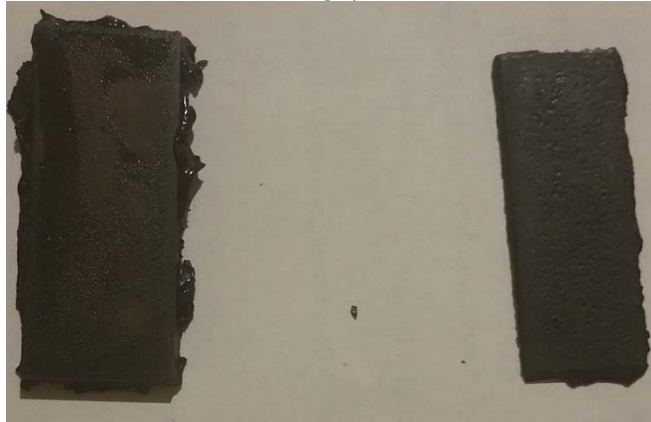
Figure 5. Day 5: Clean (left) and rusted (right) specimen before test
